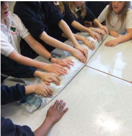
9. The hard work really begins now - with the rolling process. After 100 rolls, the felt is un-rolled then turned 45 degrees then re-rolled. This happens until the material does not pull apart when tugged.
